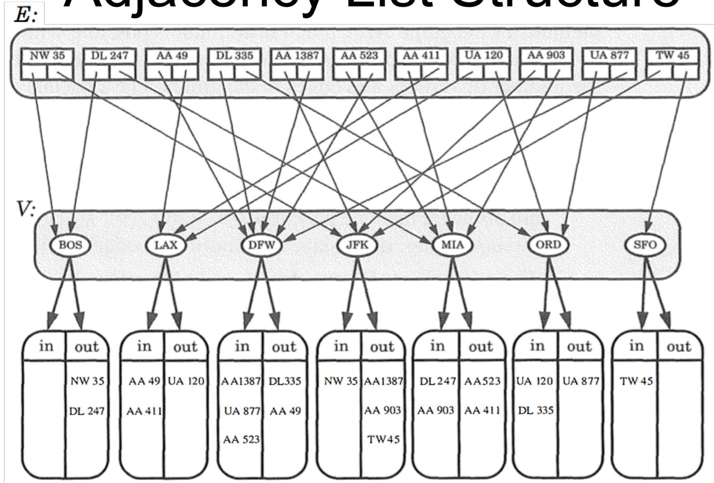
An edge list structure, where additionally each vertex object  $v$  references an incidence container which stores references to the edges incident on  $v$ .
