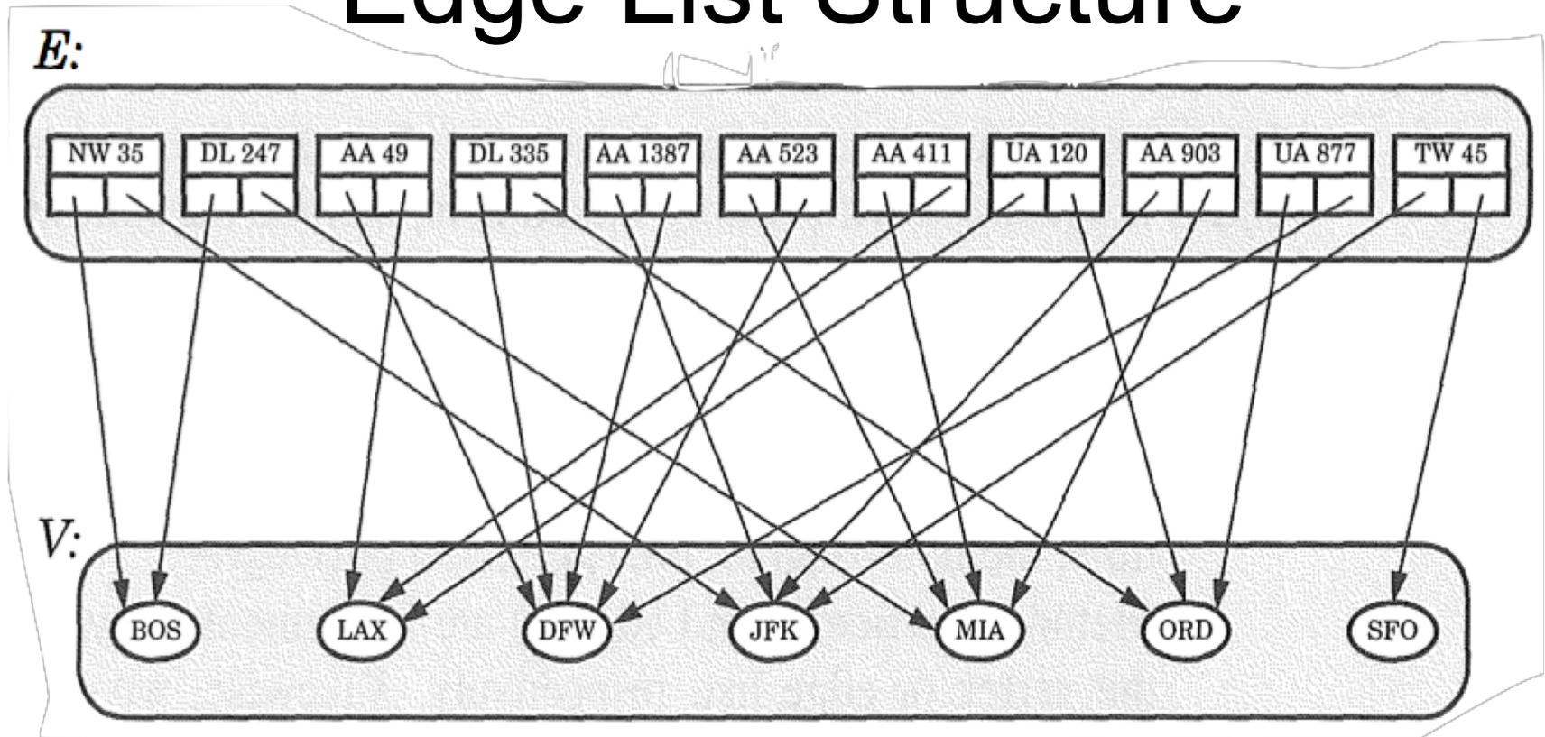
A container of edge objects, where each edge object references the origin and destination vertex object
