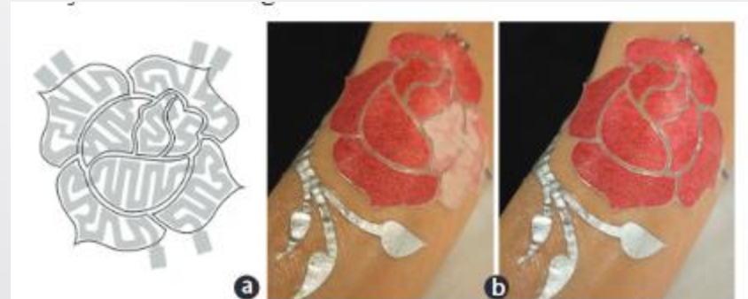
Figure 7: (a) Display with three cells. (b) A cell (right petal) is activated and turns white; when deactivated, it returns to red.
