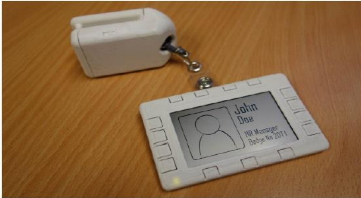
Figure 1. Prototype interactive badge and associated belt clip.
