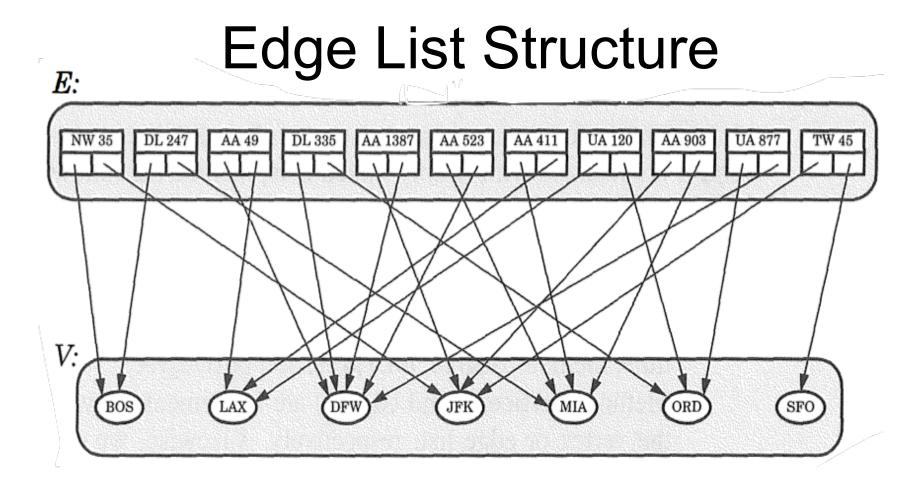
A container of edge objects, where each edge object references the origin and destination vertex object
