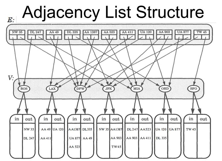
An edge list structure, where additionally each vertex object v references an incidence container which stores references to the edges incident on v.
